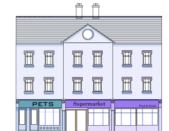
A Consistent fascia relates to the adjacent shopfront and the rest of the building
